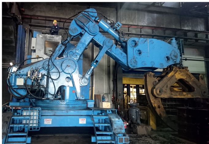
C20020 rail bound manipulator with 20 tonnes capacity
