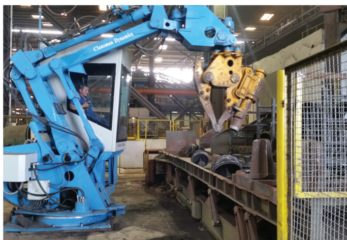
C620 manipulator with gripper mounted cannon
