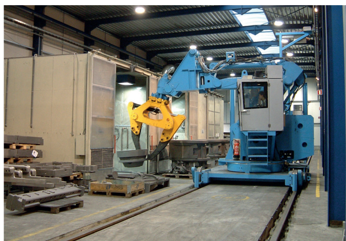
C5010 rail bound manipulator with 5 tons capacity
