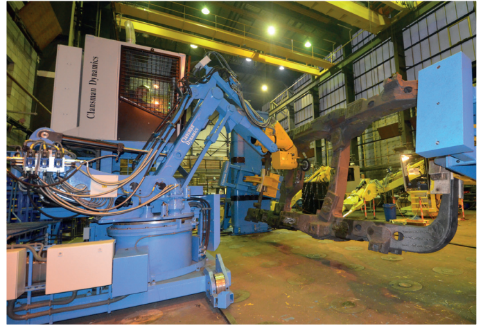
G30 Grinder in build for grinding locomotive frames
