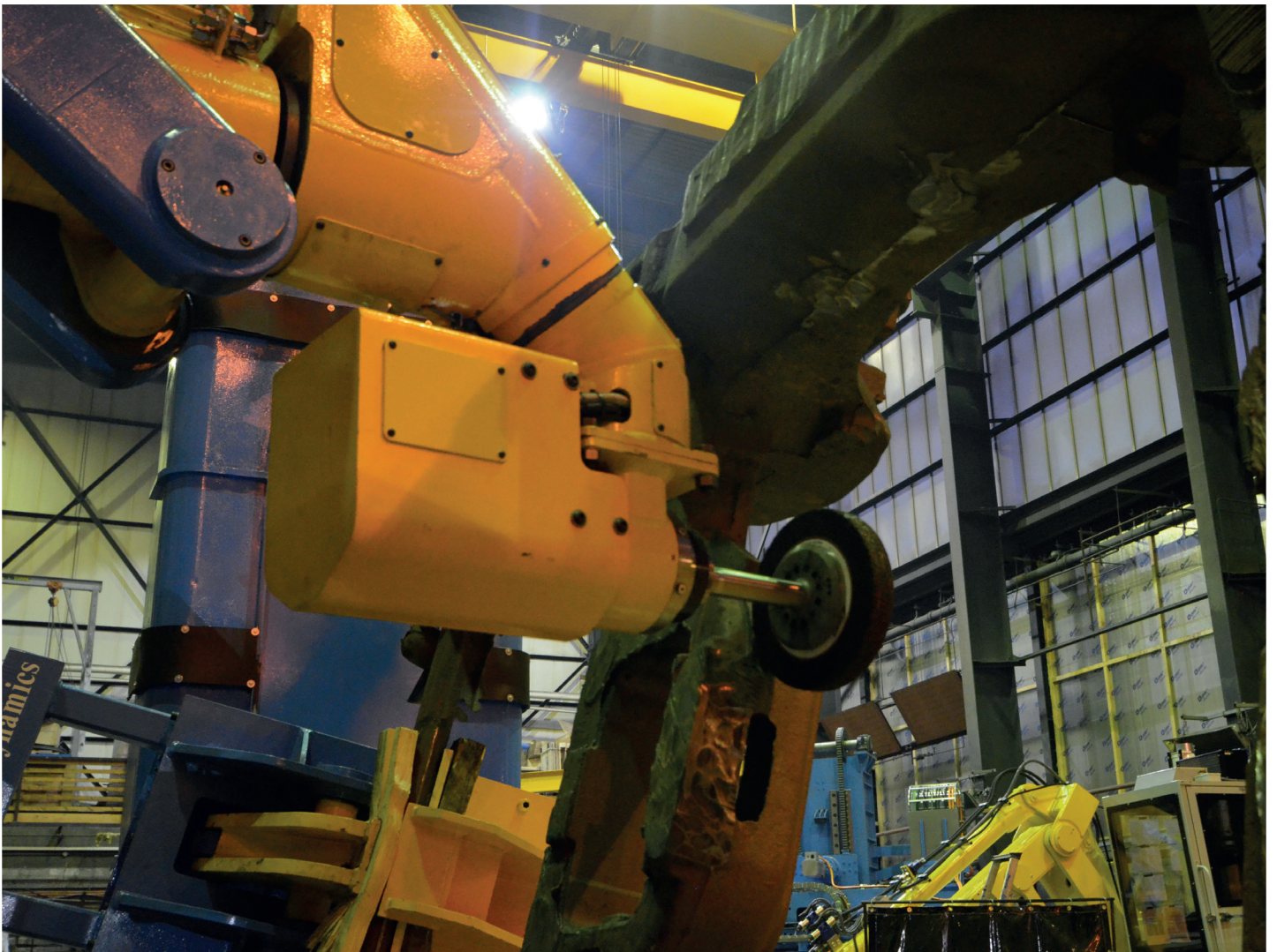
G30 Grinder has a 30 KW hydraulic spindle
