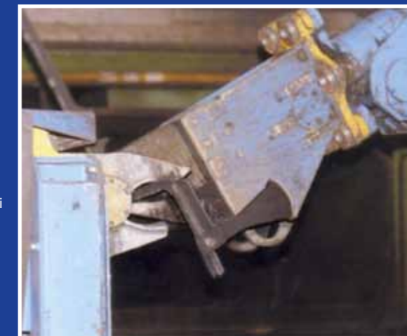
1. PB20 Powerbreaker cutting ductile iron gatings
