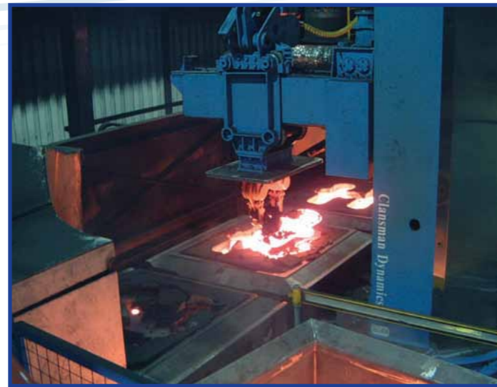
2. C410 Robot – automatic gating removal – ductile iron
