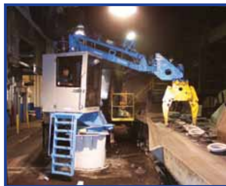
2. C620 Manipulator – sorting 600 castings per hour
