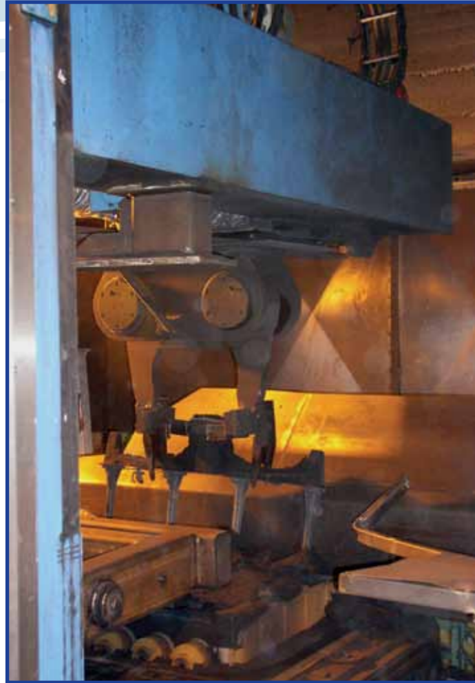
1. C4100 robot – automatic gating removal – blocks
