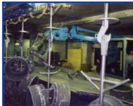
5. C620 Manipulator Loading 600 castings per hour to monorail
